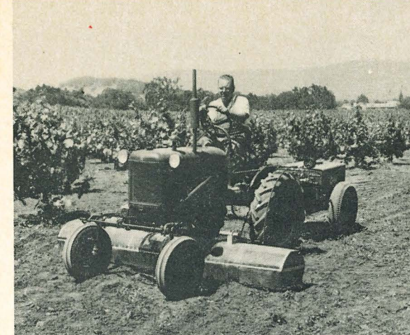
Tractor equipped with hooded boom and flooding nozzles for 2,4-D application in vineyards.
